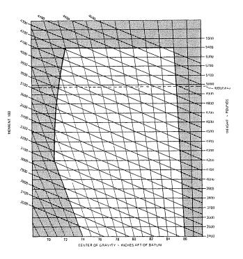
ENVELOPE BASED ON THE FOLLOWING WEIGHT AND CENTER OF GRAVITY LIMIT DATA (LANDING GEAR DOWN)
